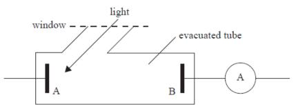
When the frequency of the light is reduced to a certain value, the current measured by the ammeter becomes zero. Explain how Einstein's photoelectric theory accounts for this observation.
